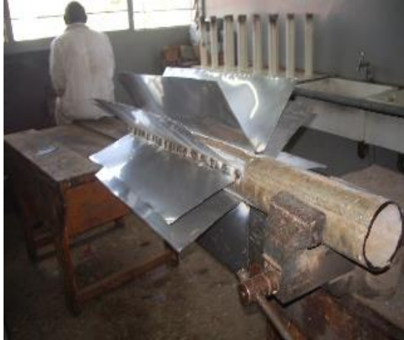
Figure 3.5 Flue pipe finned with stainless steel sheets
