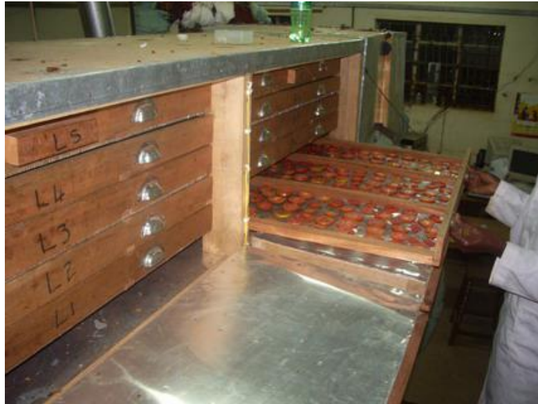
Figure 3.30 Loading of drying trays into the drying chamber.
