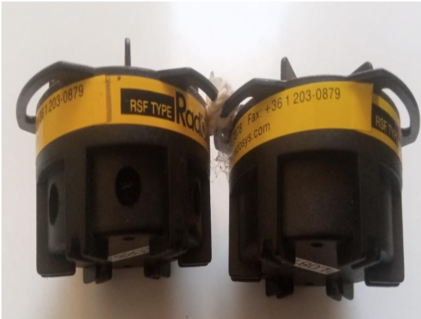
Figure 4.7: RADUET monitor pair used in this study for ^{222}\text{Rn} & ^{220}\text{Rn} concentration measurement
