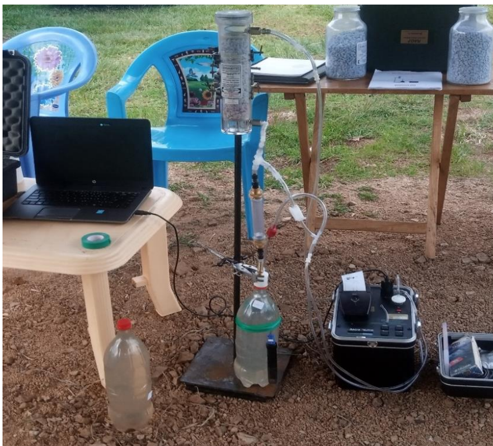
Figure 4.16: A photograph showing the big bottle technique assembly experimental setup used in this study
