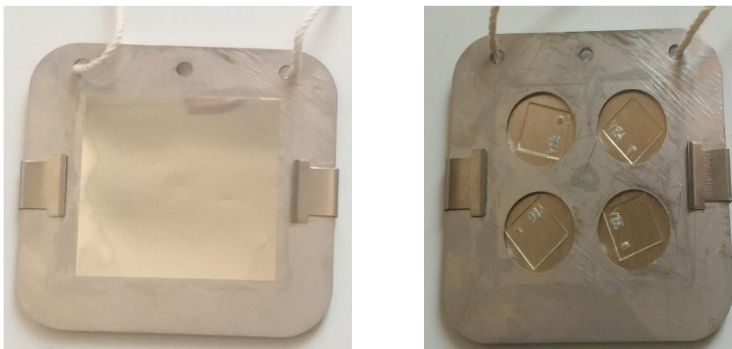
Figure 4.11: Picture of EETC Monitor used in this study for the ^{220}\text{Rn} progeny measurements
