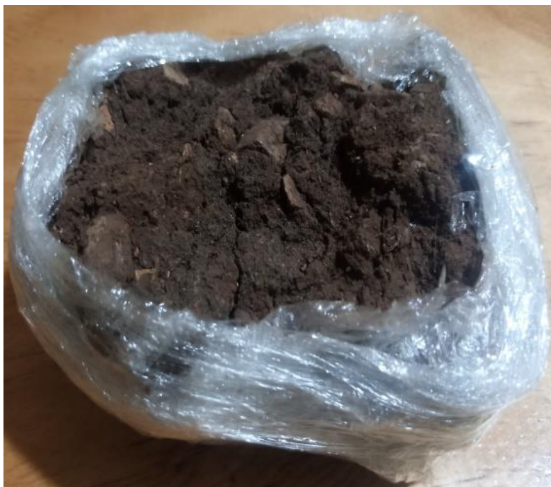
Figure 4.4: A snapshot showing pre-covered soil lump sample for the ^{222}\text{Rn} and ^{220}\text{Rn} exhalation measurement
