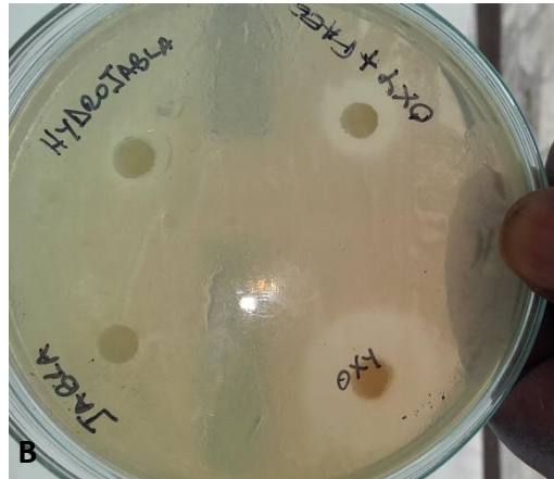
Plate 4.4: Zones of inhibition by JABLA with 8 % d -limonene, hydrogenated and oxygenated d -limonene derivatives
