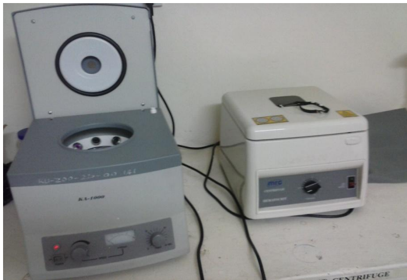
Plate b: A centrifuge used in obtaining Rabbit plasma.
