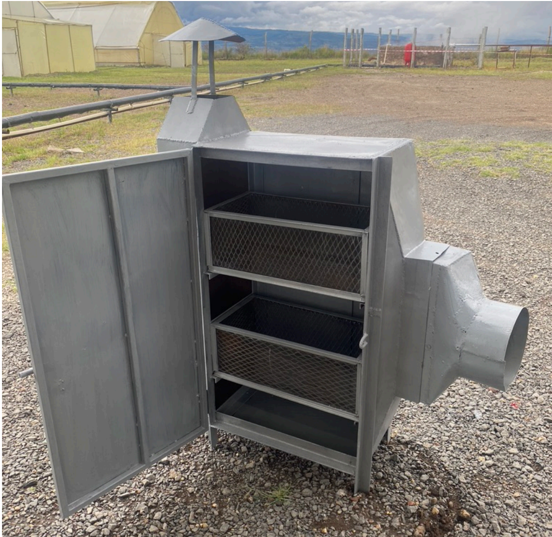
Figure 4.2: The Fabricated Geothermal Maize Dryer (Front View)
