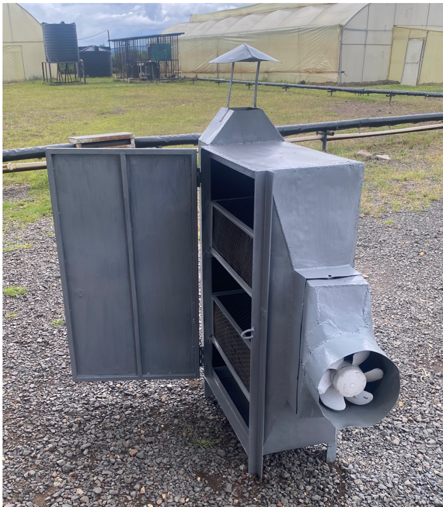
Figure 4.3: The Fabricated Geothermal Maize Dryer showing the installed fan unit but the heat exchanger is not visible (Side View)
