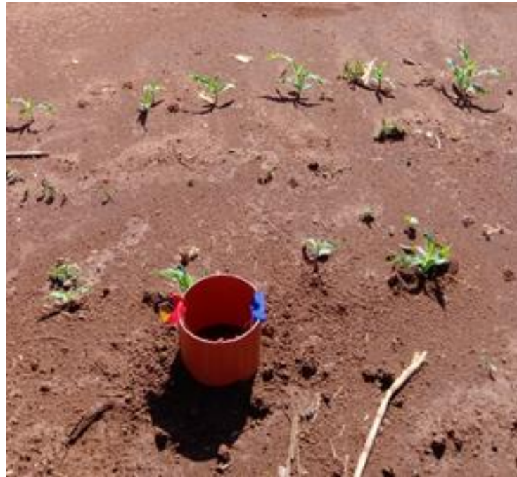
Plate 3.3 In-situ ion exchange resin incubation for nutrient mineralization assessment.
