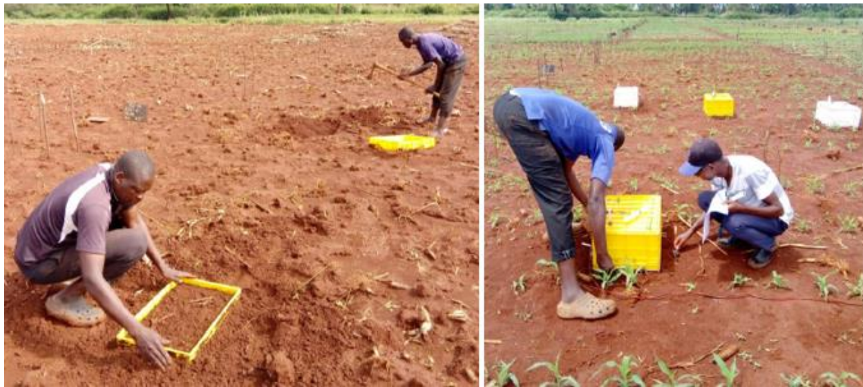
Plate 3.2. Setting up of chamber bases and in-field collection of greenhouse gases
