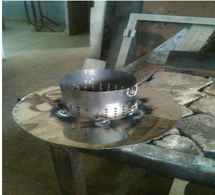
The cathode attached to the bottom lid before welding to the main body
