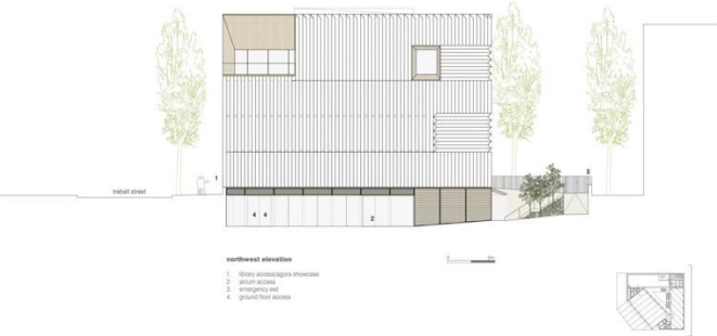
Elevation showing ramps and staircase used for access of the building by users. Source: Metalocus
