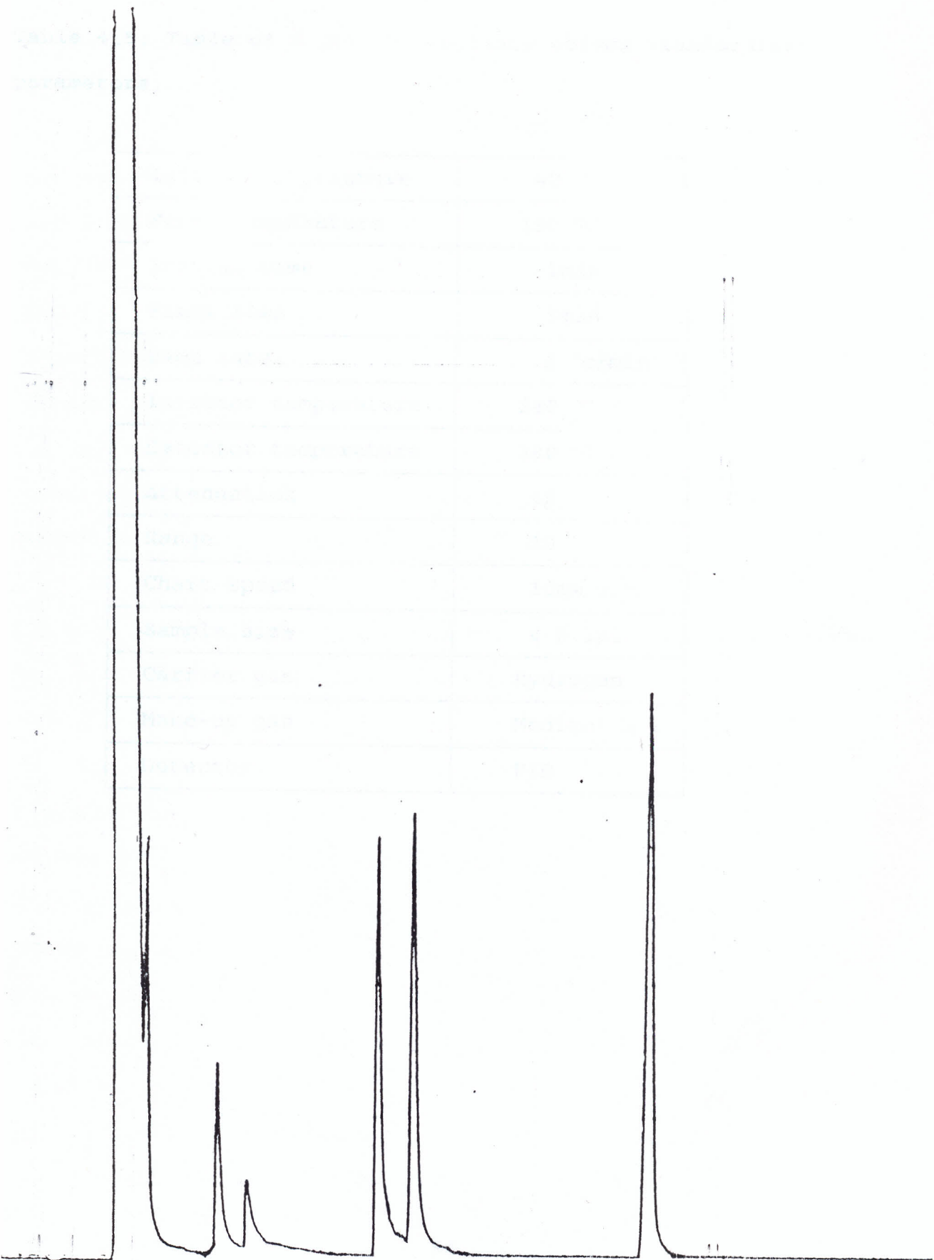
Fig. 4.7 : Sample of peak obtained when using H_2 as carrier gas and N_2 as make up gas.
