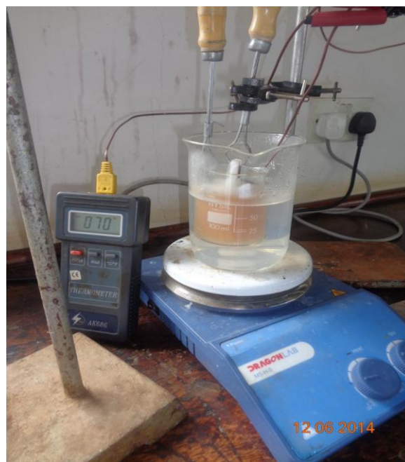
Figure 1 – Setup for chemical bath deposition used in depositing In(OH)_xS_y
