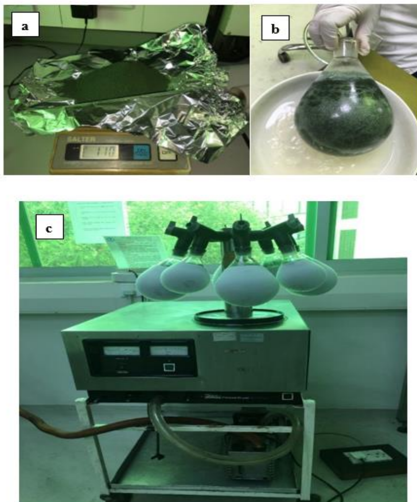
Figure 3.2 (a) Weighing of Spirulina (b) Coating round bottom flask with spirulina extract using dry ice put in acetone (c) Freeze drying of spirulina extract (Photos by author)
