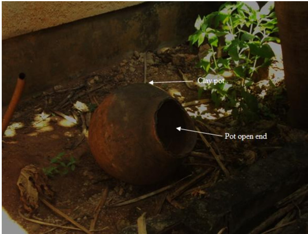
Figure 4: A picture of a clay pot used to sample adult mosquitoes outdoor
