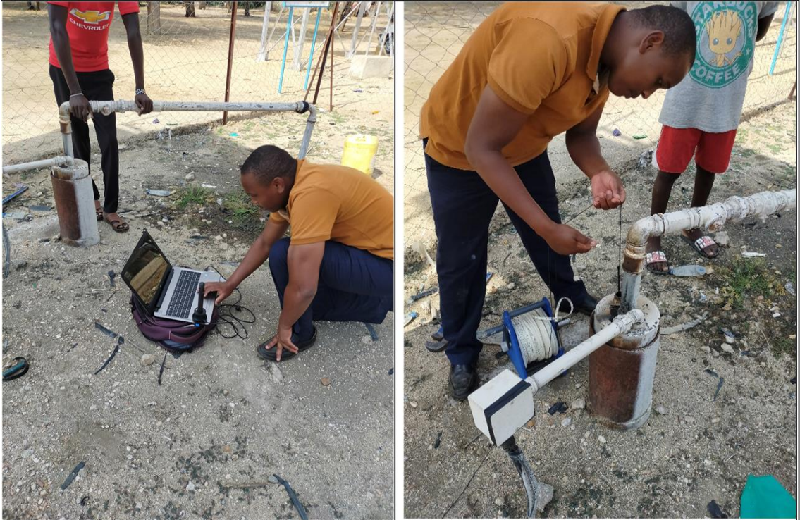
Plate 3.2: Borehole Water Level Measurement
