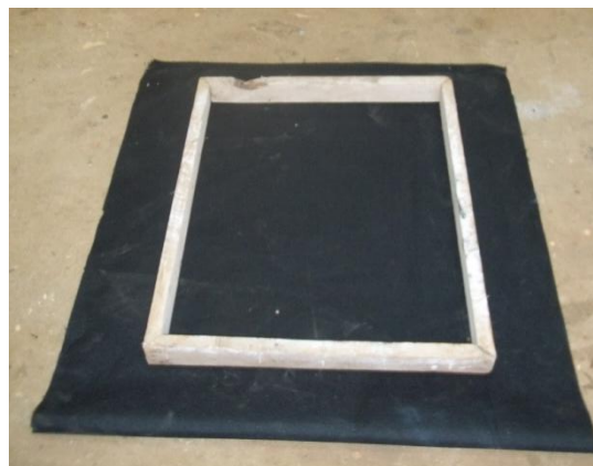
Plate 31: Centering the Canvas on the frame. Source: Researchers photo
