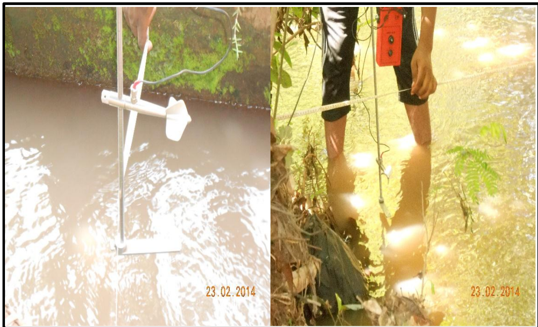
Plate 3.1: Discharge measurement using Current Meter (Source: Author, 2014)
