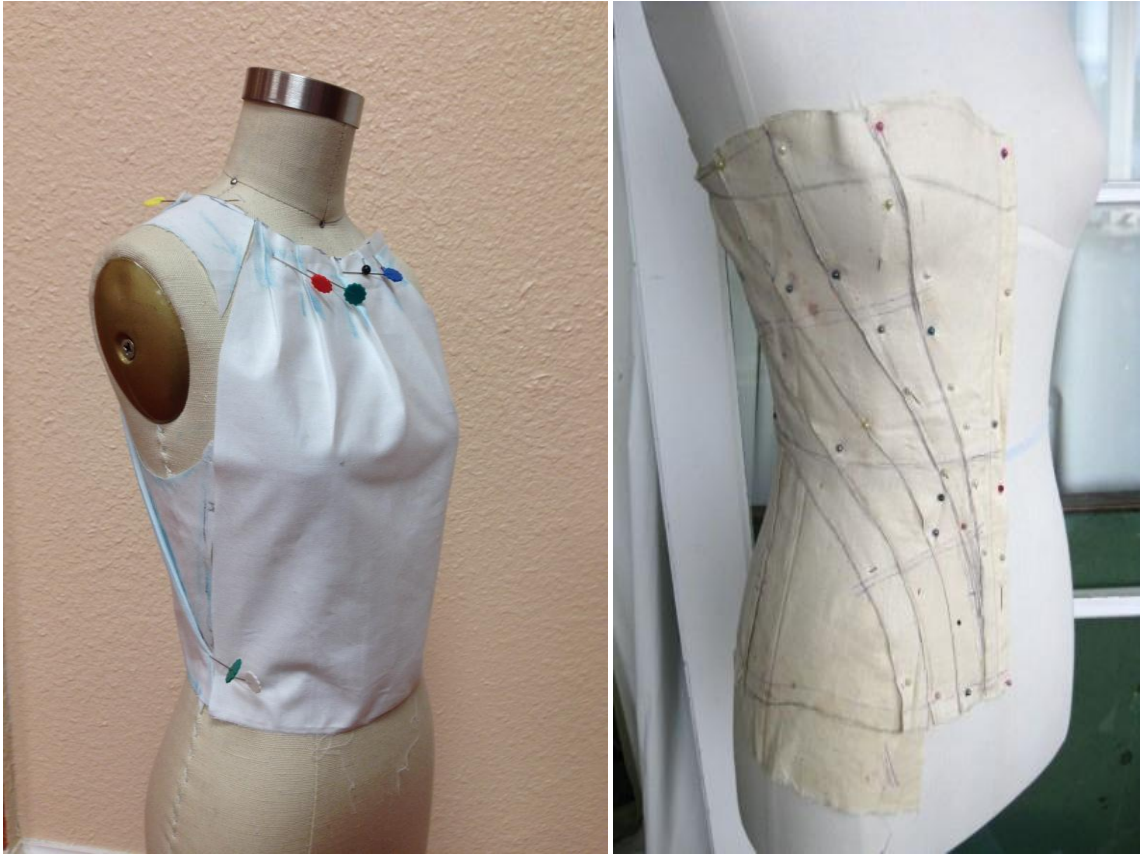
Figure 2.1: Pattern development by 'real' fabric draping for design
