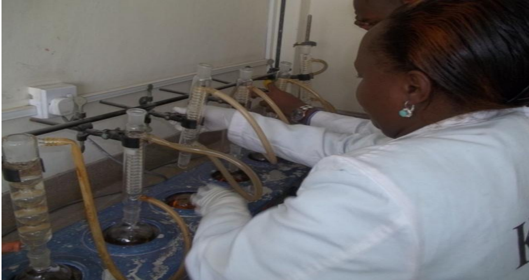
Plate 3.12: Reflux COD measurement apparatus
