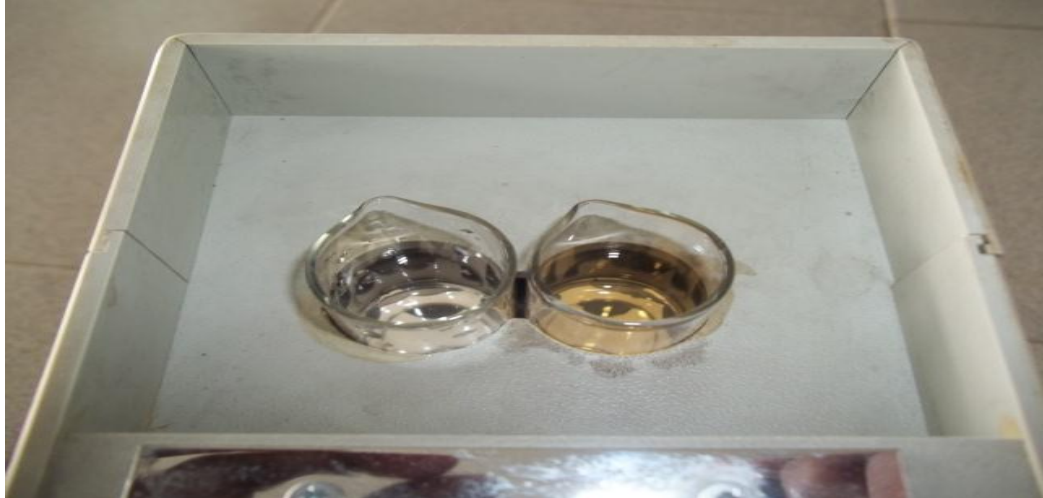
Plate 3.10: Lovibond colour measurement apparatus
