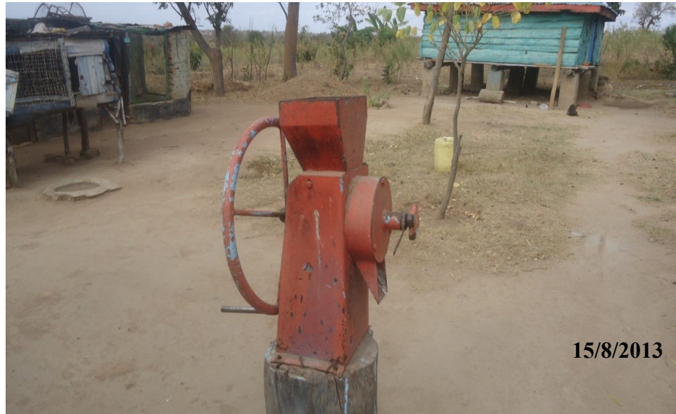
Plate 4.5: Grinding equipment used in post-harvest processing of Maize into smaller grains ( Nzenga ) among some households in Wote
