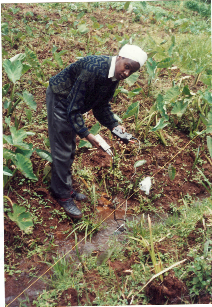
Plate 6: TDS and pH meters. (The meter probes are in the river. Water temperature was also read from the two meters).
