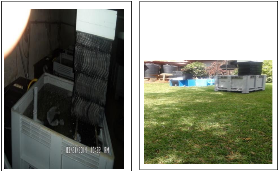
Plate 3.1: A & B) Photos of a recirculated aquaculture system(RAS) with an inbuilt bio filter, an aerator and a degassing unit at Jambo fish Farm
