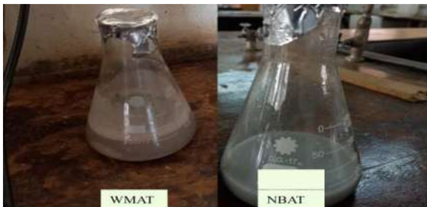
Figure 4.32 The WMAT solutions resulting from WMAT and NBAT synthesis prior to centrifugation.
