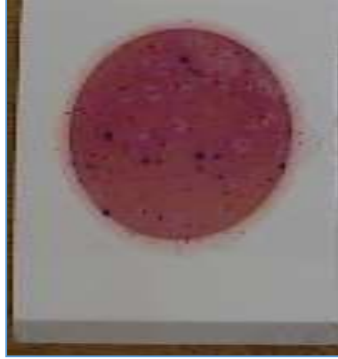
Figure 2.3 A used incubated petrifilm showing the E. coli and fecal coliform bacteria colony forming units (CFU).
