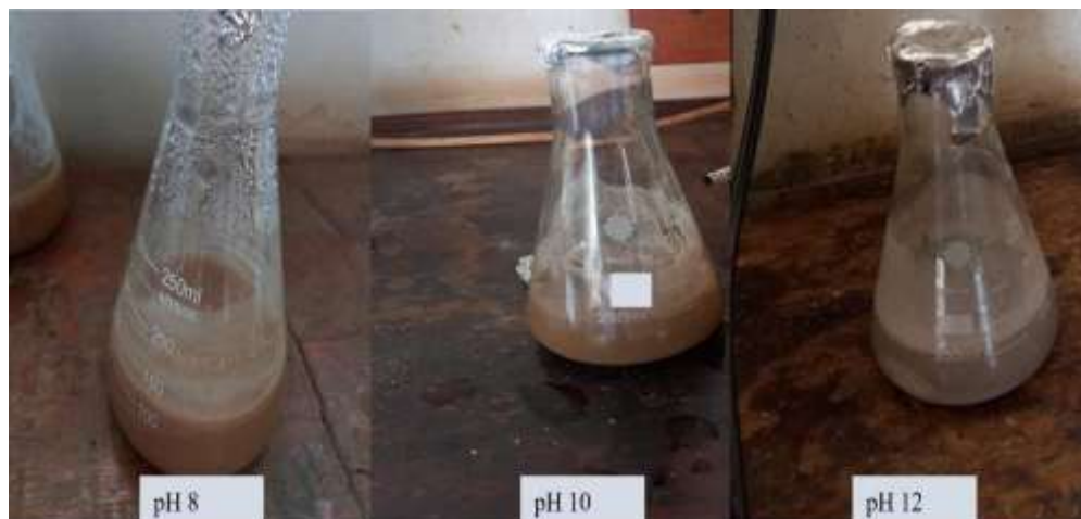
Figure 4.29 The WMAT solutions resulting from optimization at pH 8, 10, and 12 prior to centrifugation.
