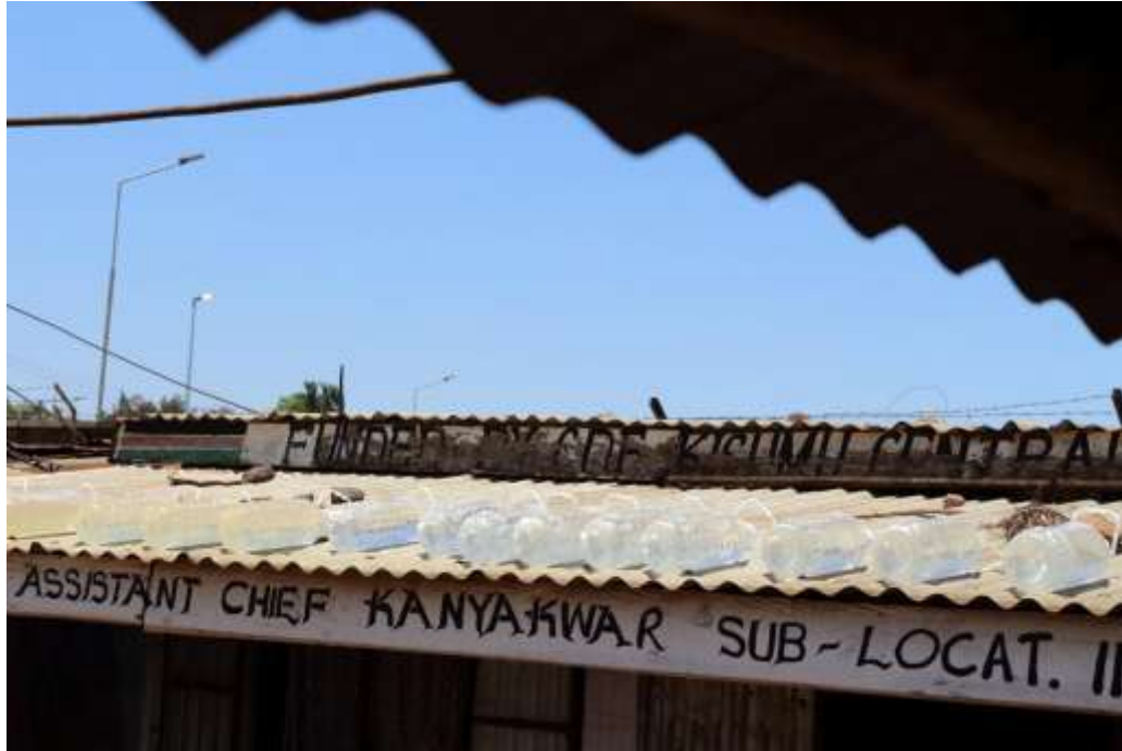
Figure 3.2 SODIS treatment set-up.
