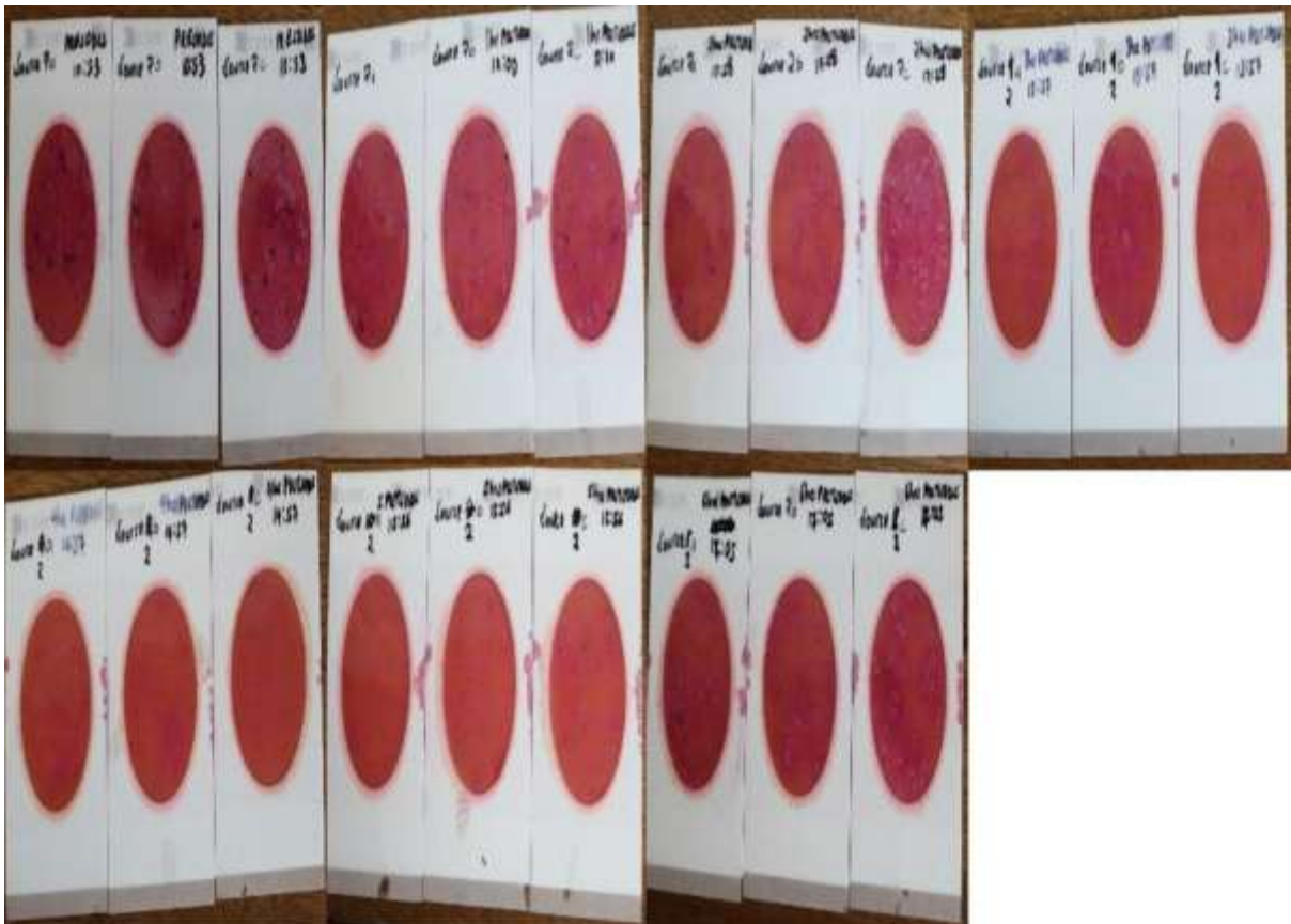
Figure 4.15 Incubated Petrifilms for water samples obtained from zone II during treatment: pre to post-SODIS.
