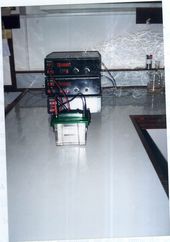
PLATE 1: SDS- PAGE equipment BIO- RAD mini- protean ® II 2000 Alfred Nobel Drive Hercules, CA 94547 U.S.A.,
