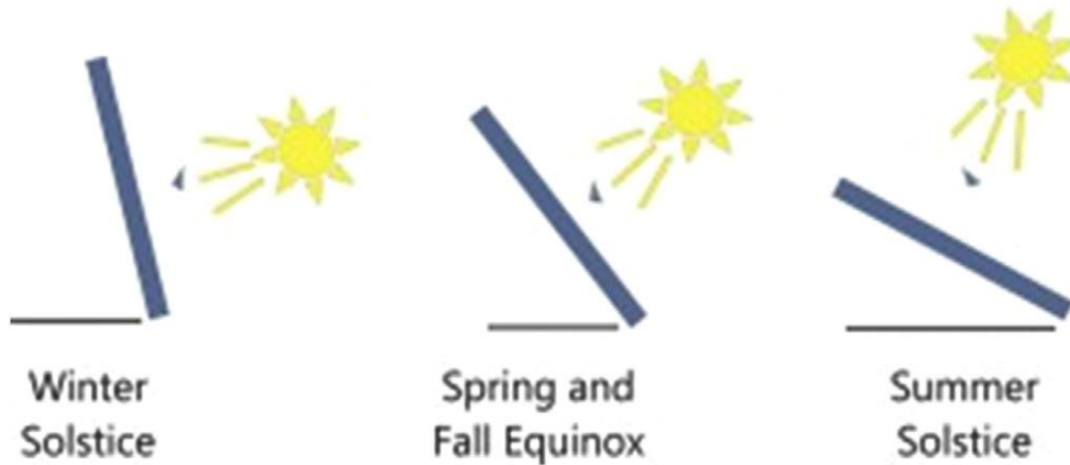
Figure 2.8: Seasonal tilt angles for solar PV system (Babatunde et al. , 2018)
