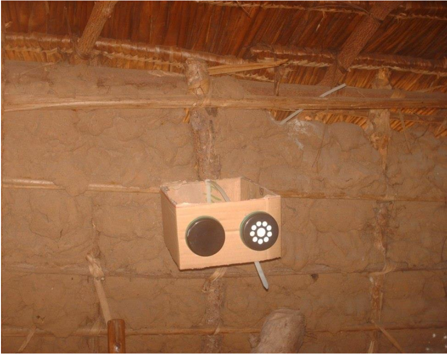
Plate 4.2: Twin canisters deployed in a dwelling in Mrima Hill
