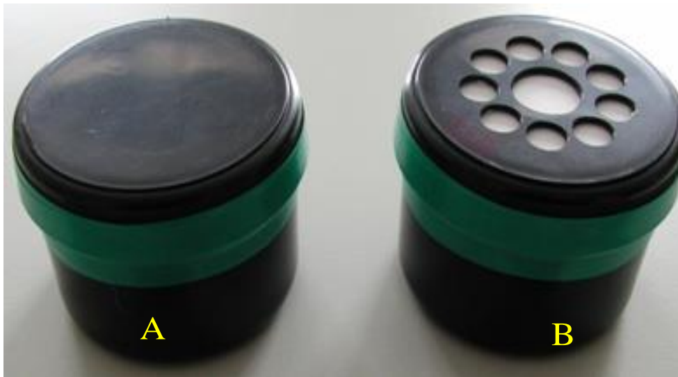
Plate 4.1: A picture of twin canisters fitted with CR-39 used for discriminative measurements of radon and thoron in this study
