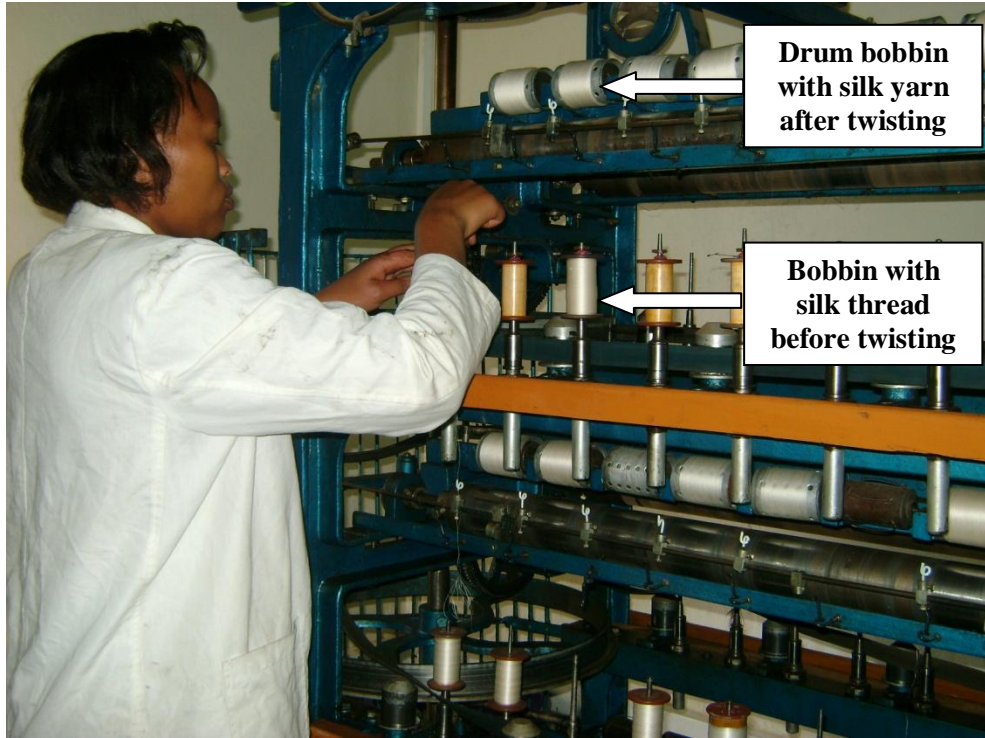
Plate 3.7 Silk Doubling/Tripling Unit
