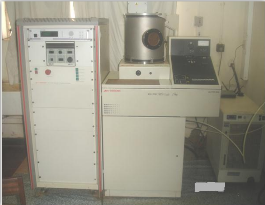
Fig. 4.1: Edwards Auto 306 Magnetron Sputtering and Evaporation equipment
