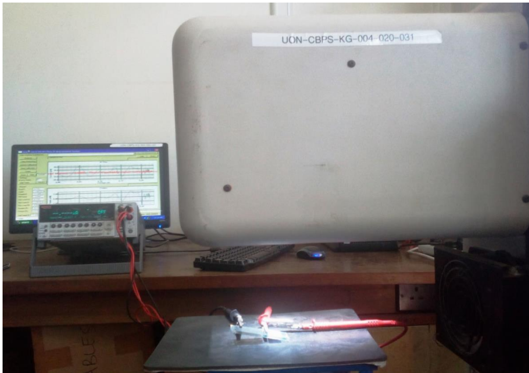
Fig. 4.9: Set – up for I-V characterization
