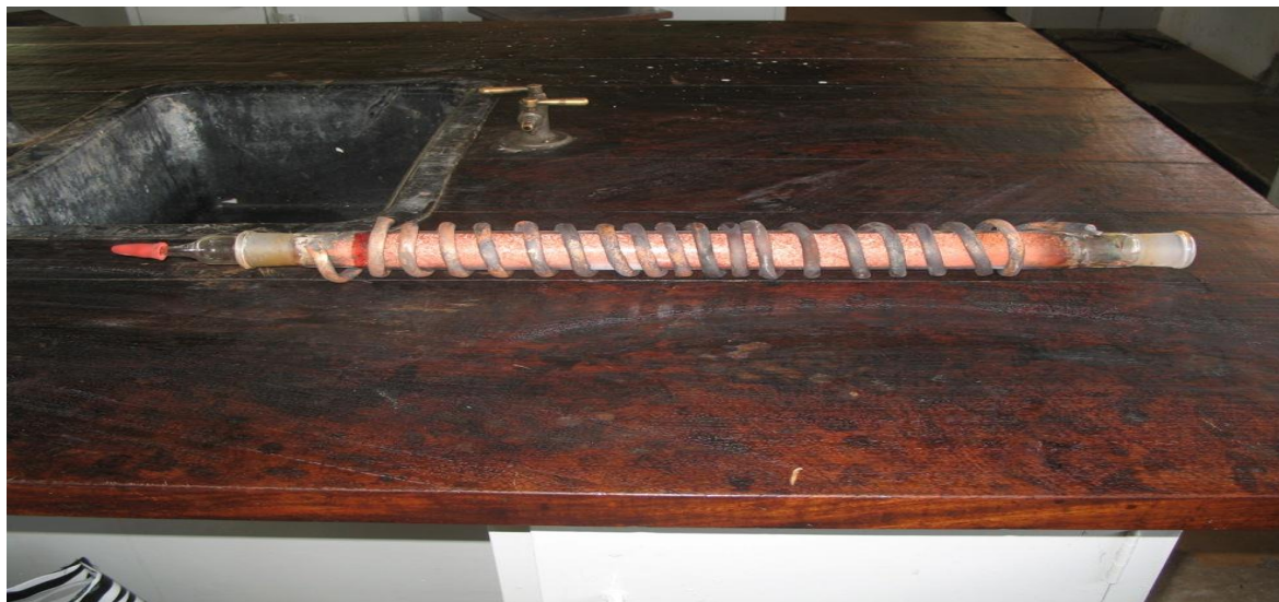
Fig. 3. 2 Glass column wound with copper wire
