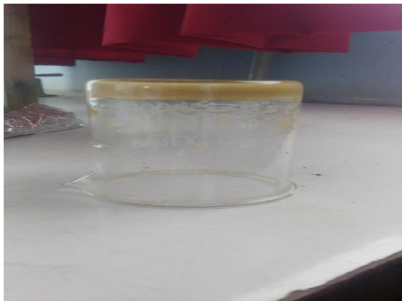
Plate 3.2: Superabsorbent hydrogel from carboxymethylcellulose crosslinked with ethane-1,2-diol seen stuck at the bottom of the beaker
