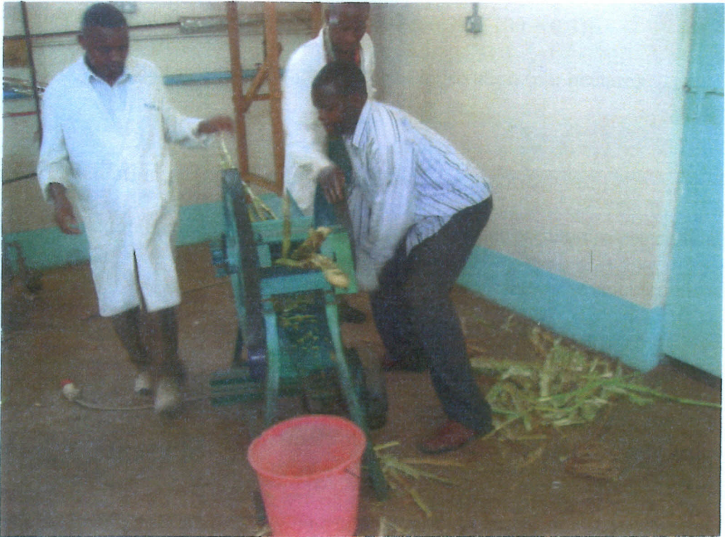
Figure 3.1: The 3-roller mill crushing equipment (locally made in Kenya)
