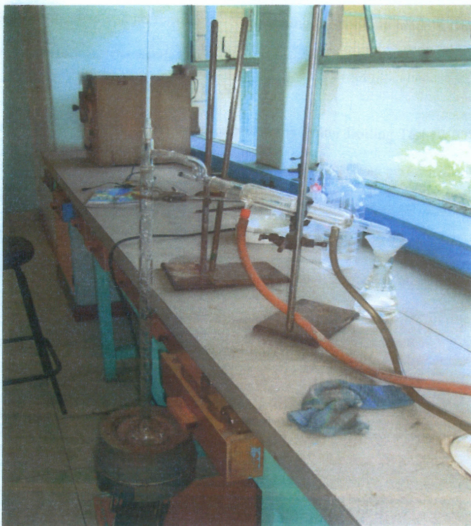
Figure.3.4: Fractional distillation of ethanol set-up
