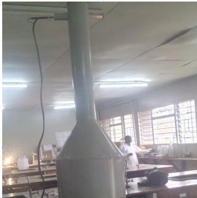
Figure 3.10 Exhaust hood and the connected probe
