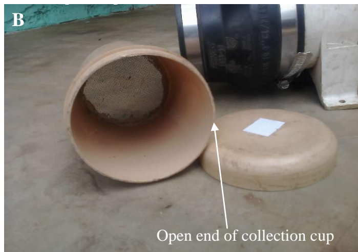
Figure 3: (A) Picture of the prokopack aspirator, 12V battery and plastic collection cup; (B) shows a picture of the open end of the collection cup
