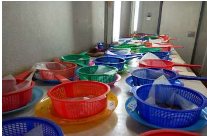
Figure 3.2: Modified Baermann technique used in the extraction of nematodes from root and soil samples. (Photograph: Nyang'au, 2018)
