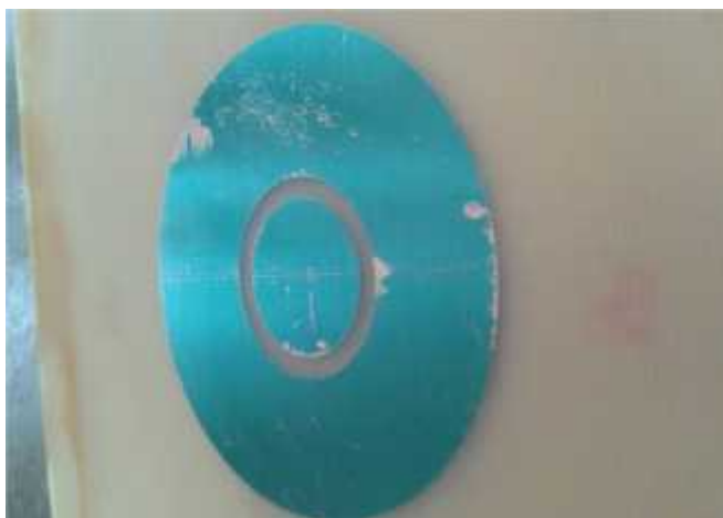
Figure 3.13: Fabricated CMPA before cleaning
