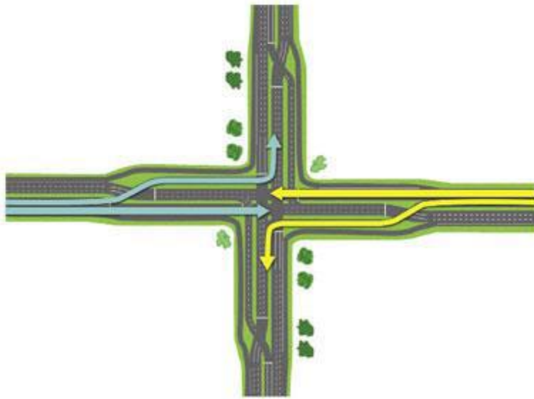
Figure 2.4: Continuous Flow Intersection (Source: Lee, 2013)
