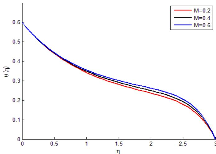
**Figure 7: Temperature representation for various values of magnetic parameter**
