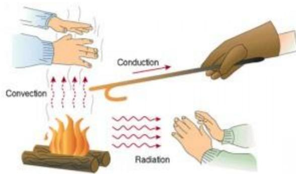
**Figure 1: Modes of heat transfer (www.spectrose.com)**
