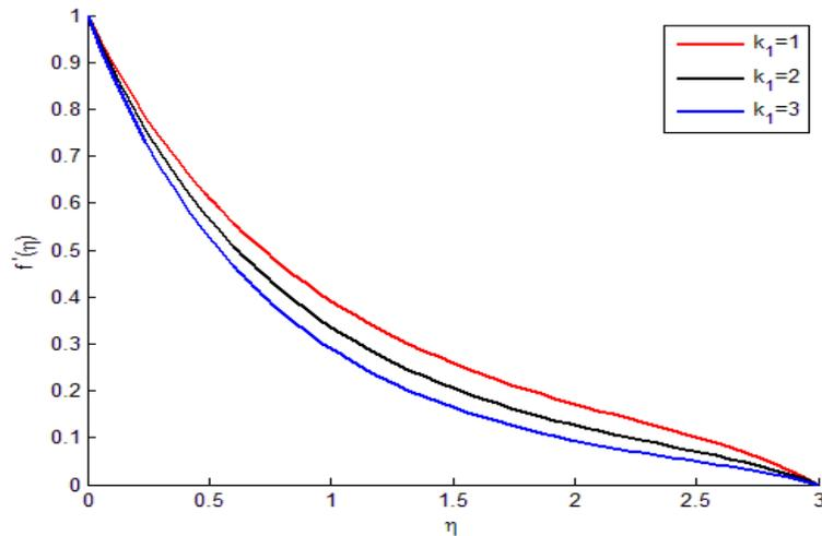
**Figure 10: Velocity representation for different values of permeability parameter**
