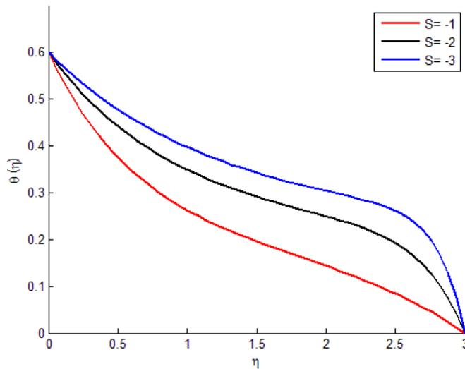
**Figure 13: Temperature representation for different values of injection**
