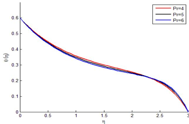
**Figure 17: Temperature representation for different values of prandtl number**
