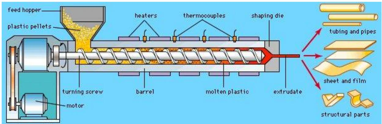
**Figure 2: An extruder ([isac.wikidot.com/polymer-extrusion-gallery](http://isac.wikidot.com/polymer-extrusion-gallery))**
