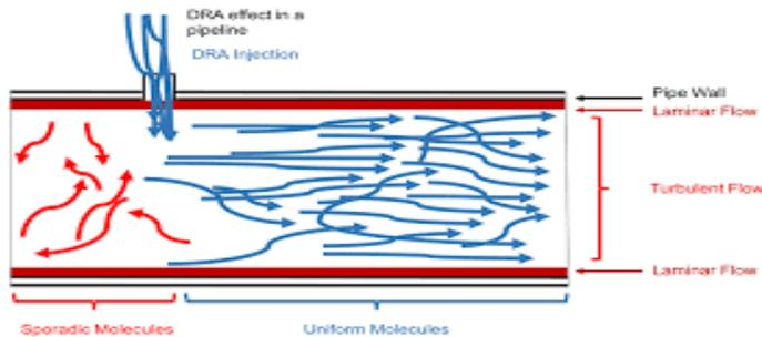
**Figure 3: Schematic diagram on the effect of DRA on the flow of fluid in a pipe**
