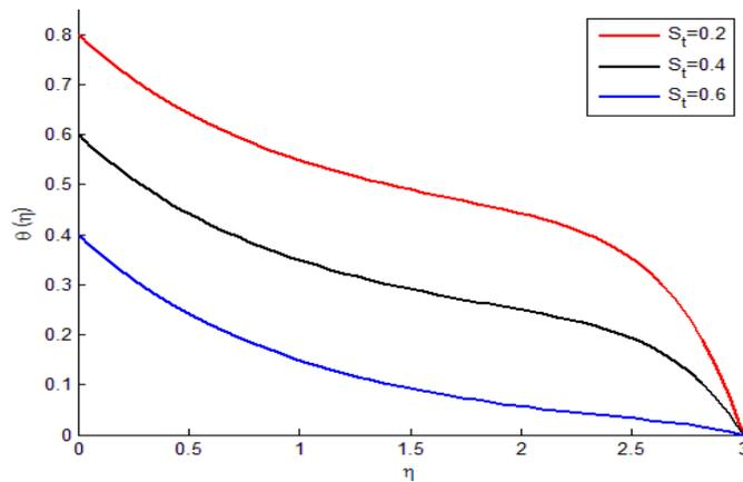
**Figure 16: Temperature representation for different values of stratification parameter**
