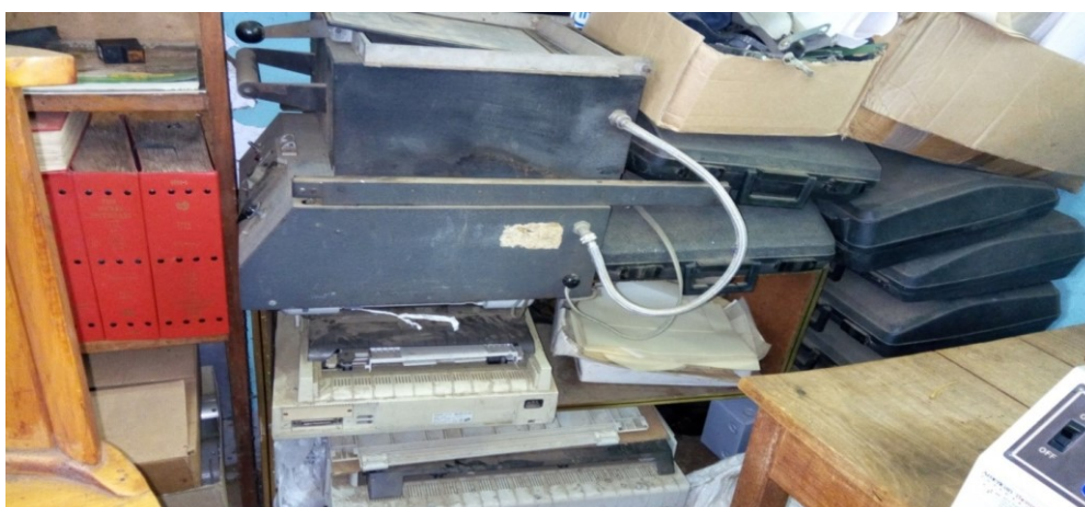
Plate 1.A: A pack of broken down thermoform machine (on top) and a perforating machine below it at study site A
