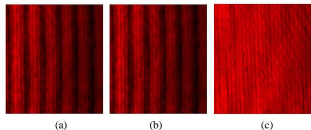
**Figure 4. Sample interferograms captured by CCD for piston ring 2. The interferograms were characterized by geometrical variation as temperature increased. (a) The interference fringes are linear at  $25^{\circ}\text{C}$ ; (b) The interference fringes are curved at  $35^{\circ}\text{C}$ ; (c) The interference fringes appear compressed at  $100^{\circ}\text{C}$ .**
