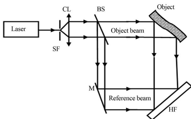
**Figure 1.** Schematic illustration of holographic recording set-up. SF is the spatial filter, CL is the collimating lens, BS is the beam splitter, HF is the holographic plate and M is reflecting mirror.
