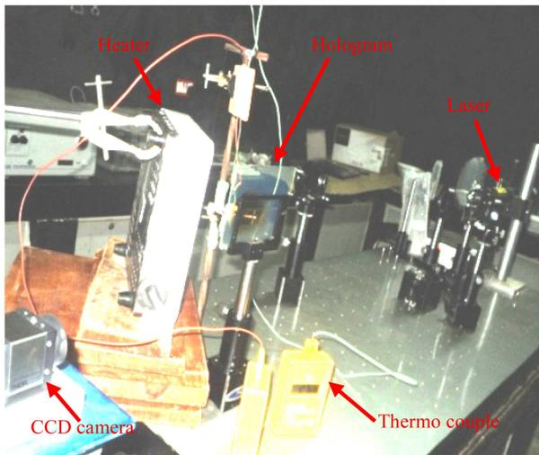
**Figure 2. Real time holographic interferometric set up. The developed plate was replaced on the holder and the object subjected to heating. Using a CCD camera the generated interferograms were captured for analysis.**
