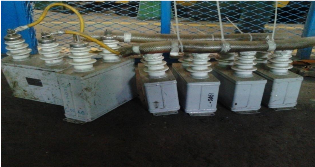
Photo image 2: E-waste from AC Electrolytic capacitors (photo series by Duncan Aliero Muhani)
