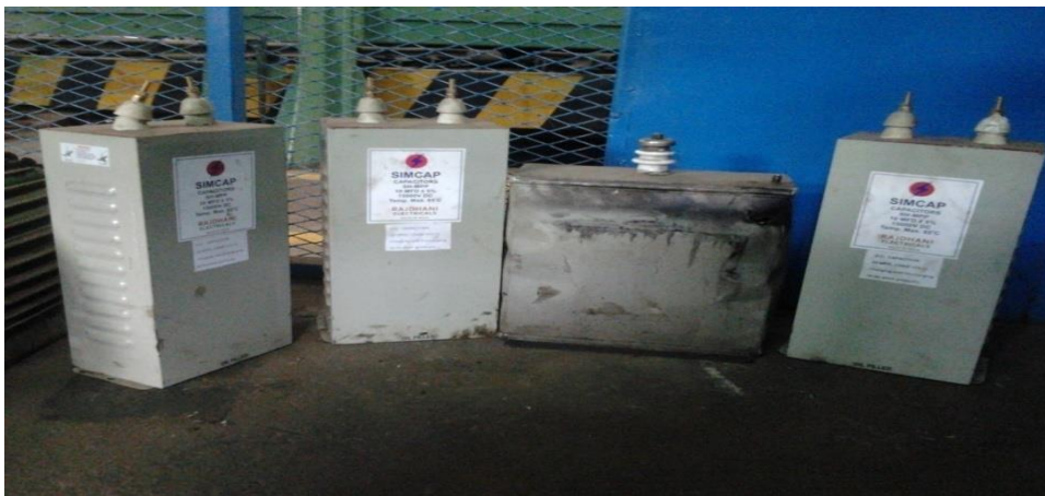
Photo image 3: E-waste from counterfeits AC oiled field capacitors (photo series by Duncan Aliero Muhani)
