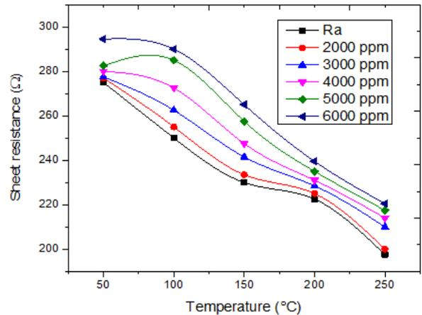
Figure 11. Sheet resistance versus temperature for the as annealed Pd-F:SnO<sub>2</sub> thin film.
