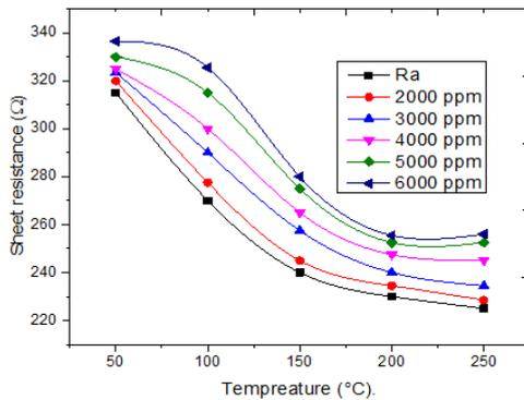
Figure 10. Sheet resistance versus temperature for the as prepared Pd-F:SnO<sub>2</sub> thin films.
