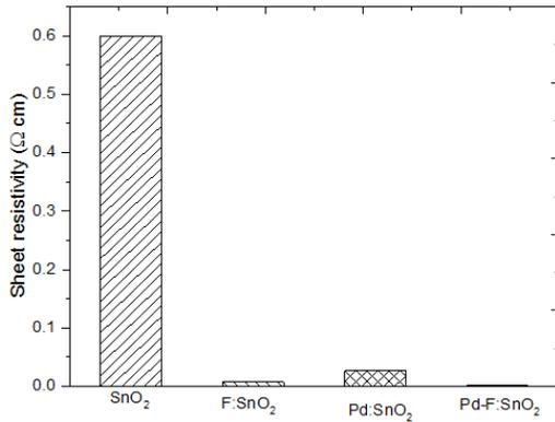
Figure 8. Sheet resistivity characteristics of SnO<sub>2</sub>, F:SnO<sub>2</sub>, Pd:SnO<sub>2</sub> and Pd-F:SnO<sub>2</sub> thin films
