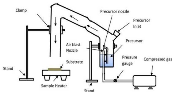
Figure 1. Spray pyrolysis experimental set up.
