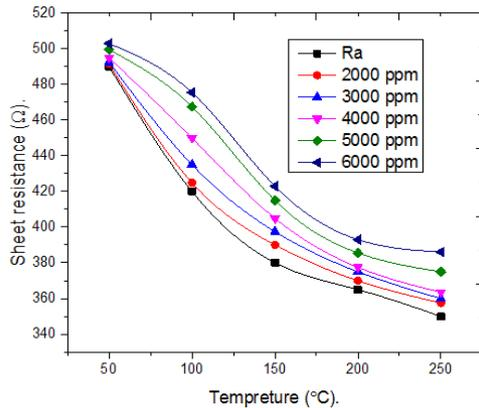
Figure 12. Sheet resistance versus temperature for the passivated Pd-F: SnO<sub>2</sub> thin film.
