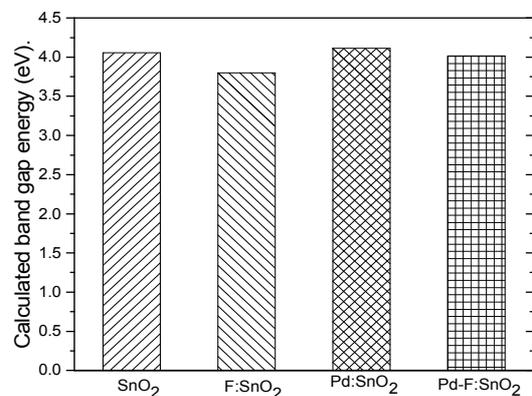
Figure 7. Calculated band gap energy for as prepared and doped SnO<sub>2</sub> thin films.
