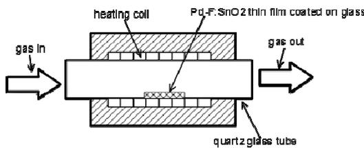
Figure 3. Horizontal tube furnace for annealing and passivation.
