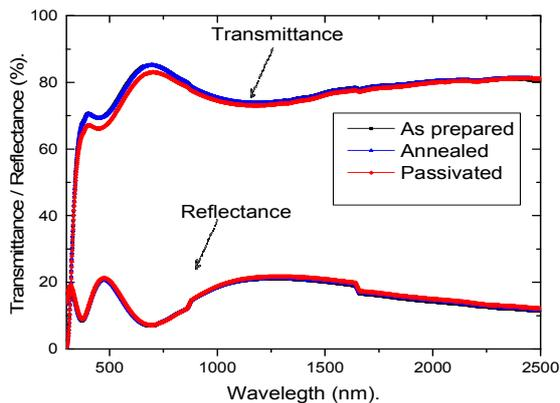
Figure 6. Transmittance and reflectance spectra for as prepared, as annealed and passivated Pd-F: SnO<sub>2</sub> thin films
