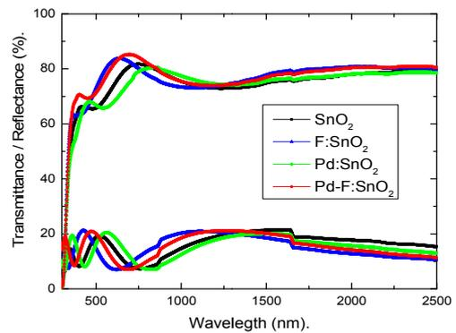
Figure 5. Transmittance and reflectance spectra for doped SnO<sub>2</sub> thin films
