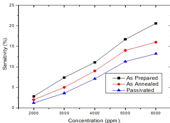
Figure 13. Sensitivity versus CO<sub>2</sub> concentration (ppm).
